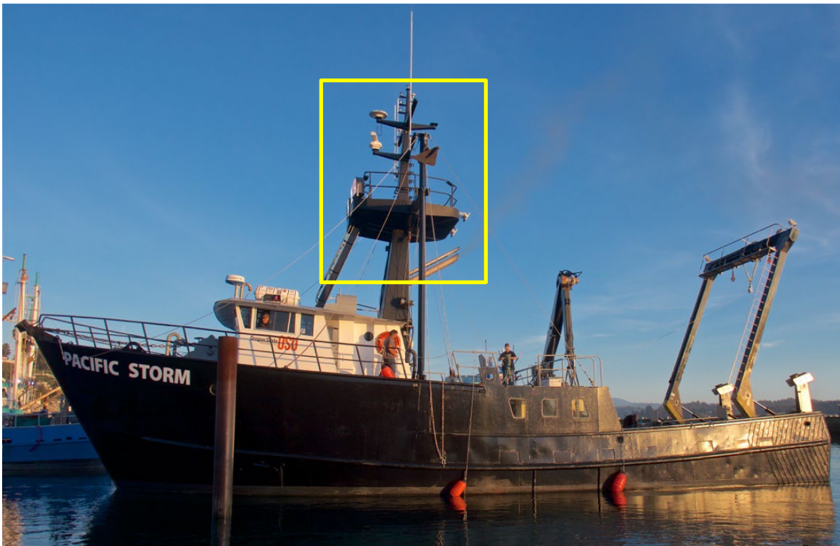
FIGURE 4. R/V PACIFIC STORM, SHOWING THE OBSERVATION PLATFORM (CROW'S NEST) OUTLINED IN YELLOW.
