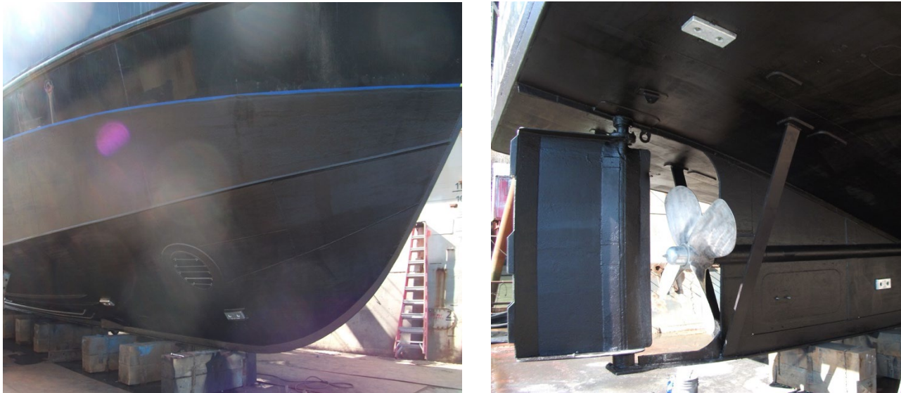
FIGURE 1. R/V PACIFIC STORM HULL, SHOWN FROM THE BOW (LEFT PANEL) AND PROPELLOR AND RUDDER (RIGHT PANEL).
